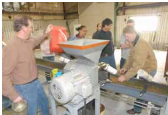
Partners Brett Earl and Logan Fisher pressing oilseeds to produce biodiesel in its Chester facility to show visiting Stone Child College students and faculty
